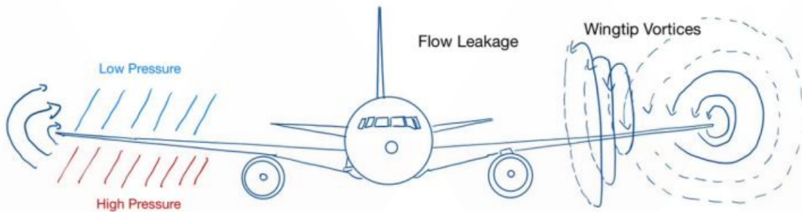
Fig.2 Wingtip Vortices Generated From Pressure Difference
